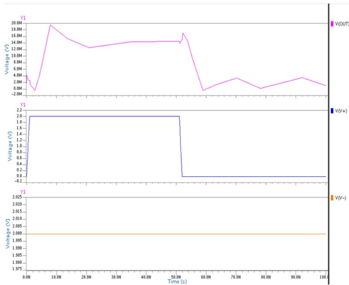
Fig 2.6. Transient Analysis of Comparator at 90nm
